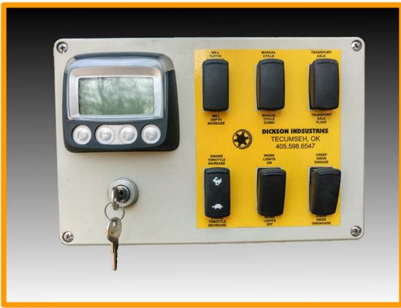
The engine control module houses the John Deere PV-101 engine monitor and display. The PV-101 not only displays current engine parameters, but also stores error codes and engine fault codes which can be read by any John Deere service technician. Also housed in the engine control module are the basic RUMBLER controls.
