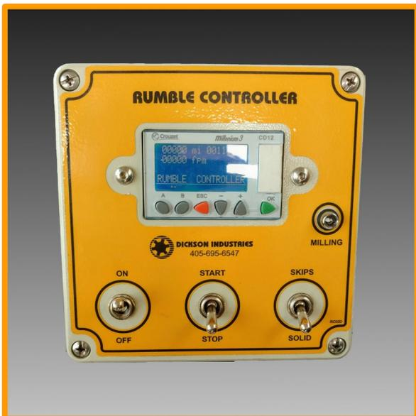
The RUMBLE CONTROLLER mounted next to the operator in the cab of the tow vehicle is used for milling rumble skips; XX feet of rumble strips followed by XX feet of skip. The pattern is easily adjustable by the operator.
